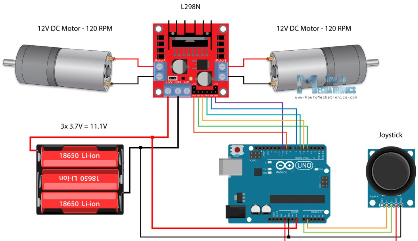
All we need is 2 DC Motors, the L298N driver, an Arduino board and a joystick for the control. As for the power supply, I chose to use three 3.7V Li-ion batteries, providing total of 11V. I made the chassis out of 3 mm tick plywood, attached the motors to it using metal brackets, attached wheels to the motors and in front attached a swivel wheel.
