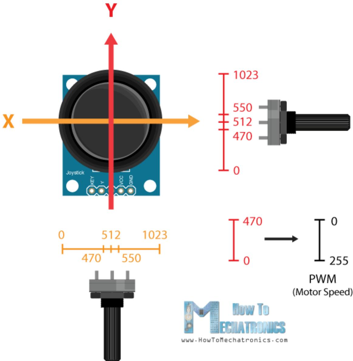
We will add a little tolerance and consider the values from 470 to 550 as center. So if we move the Y axis of joystick backward and the value goes below 470 we will set the two motors rotation direction to backward using the four input pins. Then, we will convert the declining values from 470 to 0 into increasing PWM values from 0 to 255 which is actually the speed of the motor.
