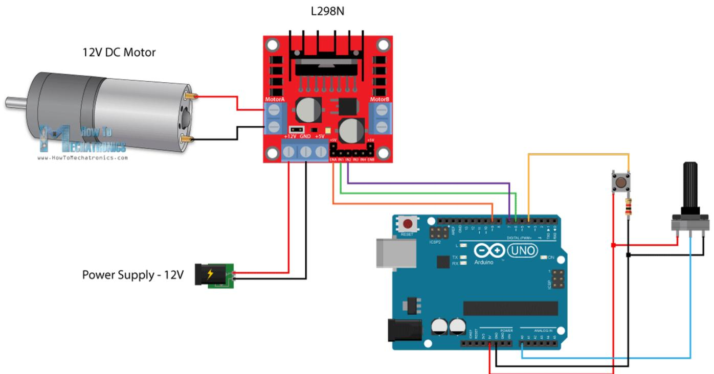
So we need an L298N driver, a DC motor, a potentiometer, a push button and an Arduino board.
