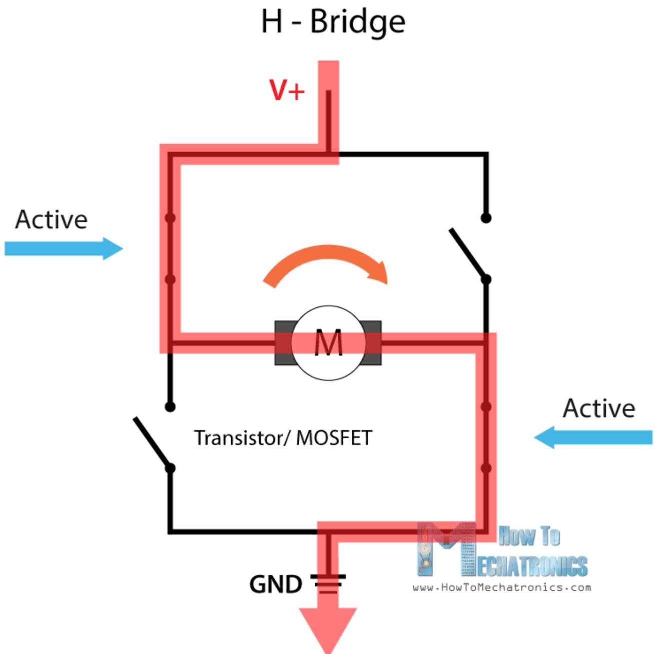
So if we combine these two methods, the PWM and the H-Bridge, we can have a complete control over the DC motor. There are many DC motor drivers that have these features and the L298N is one of them.
