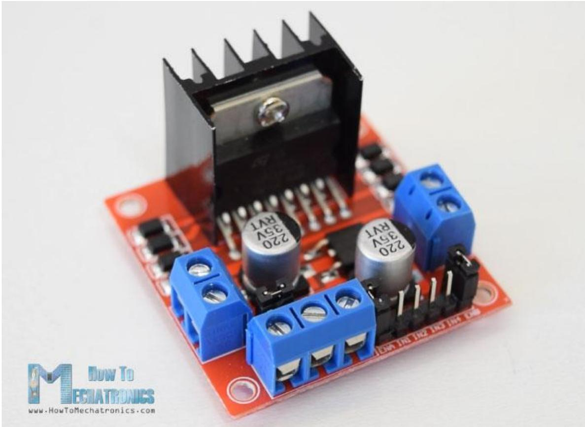
Let's take a closer look at the pinout of L298N module and explain how it works. The module has two screw terminal blocks for the motor A and B, and another screw terminal block for the Ground, the VCC for motor and a 5V pin which can either be an input or output.
