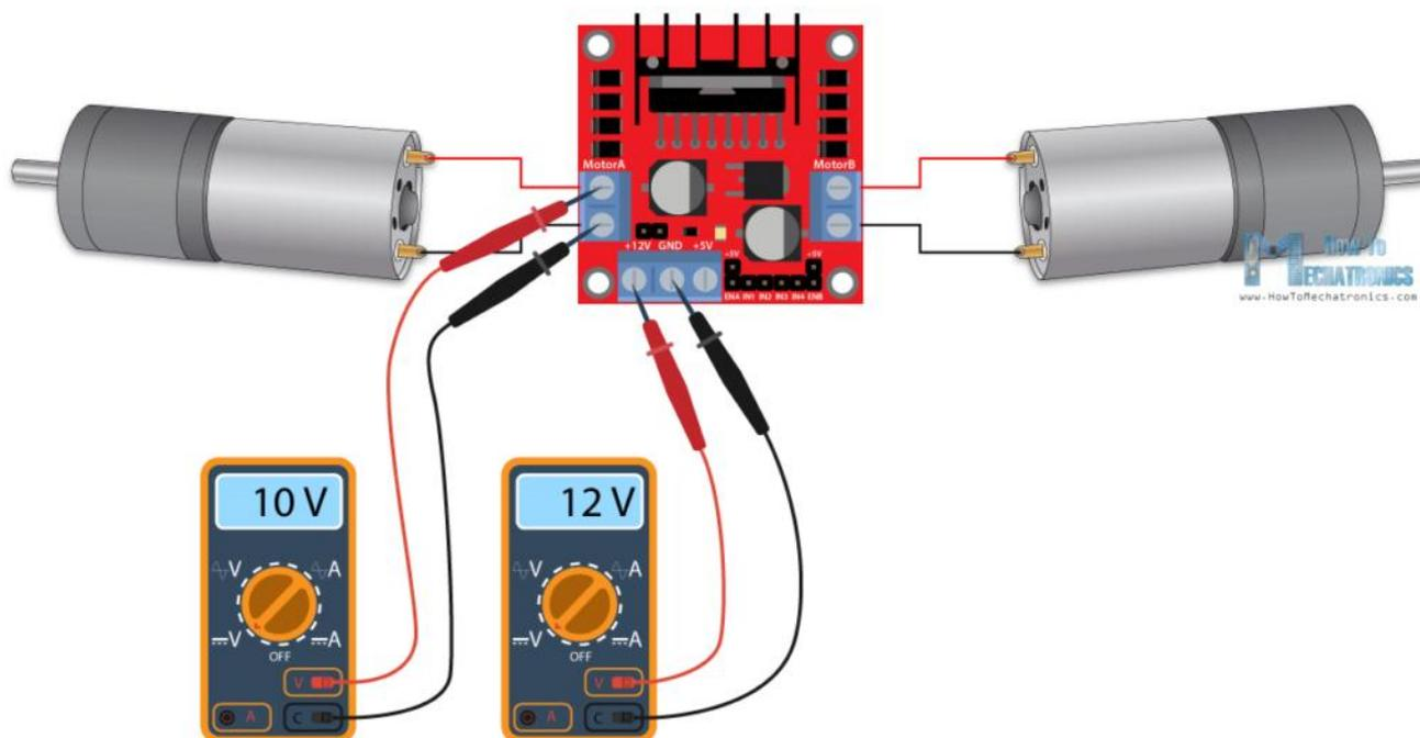
Next are the logic control inputs. The Enable A and Enable B pins are used for enabling and controlling the speed of the motor. If a jumper is present on this pin, the motor will be enabled and work at maximum speed, and if we remove the jumper we can connect a PWM input to this pin and in that way control the speed of the motor. If we connect this pin to a Ground the motor will be disabled.
