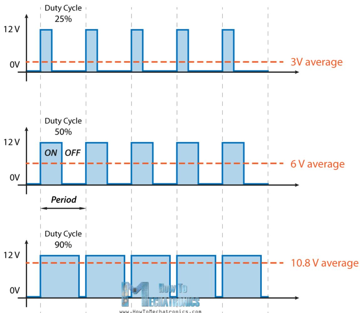
So depending on the size of the motor, we can simply connect an Arduino PWM output to the base of transistor or the gate of a MOSFET and control the speed of the motor by controlling the PWM output. The low power Arduino PWM signal switches on and off the gate at the MOSFET through which the high power motor is driven.
