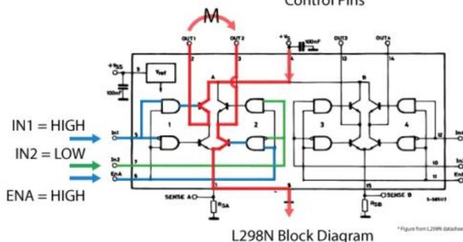
Next, the Input 1 and Input 2 pins are used for controlling the rotation direction of the motor A, and the inputs 3 and 4 for the motor B. Using these pins we actually control the switches of the H-Bridge inside the L298N IC. If input 1 is LOW and input 2 is HIGH the motor will move forward, and vice versa, if input 1 is HIGH and input 2 is LOW the motor will move backward. In case both
