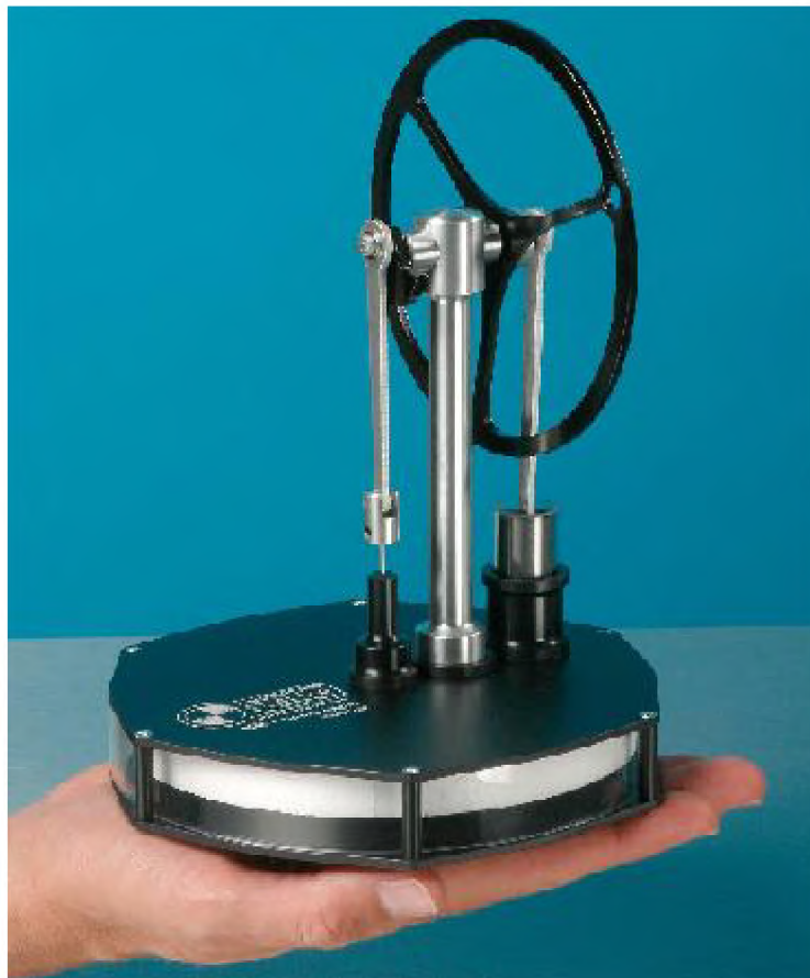
Fig(30): Dr Senft's "Heat of your Hand" engine design. A Model MM-7 Stirling engine made by the American Stirling company.
