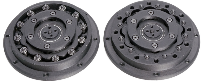
Fig. 1: Cycloidal drive prototypes: Pinwheel (left) and non-pinwheel (right) designs, with lower housing parts removed.
